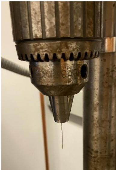
Figure 8: K-wire inserted into the tip of the drill press for the polishing procedure
