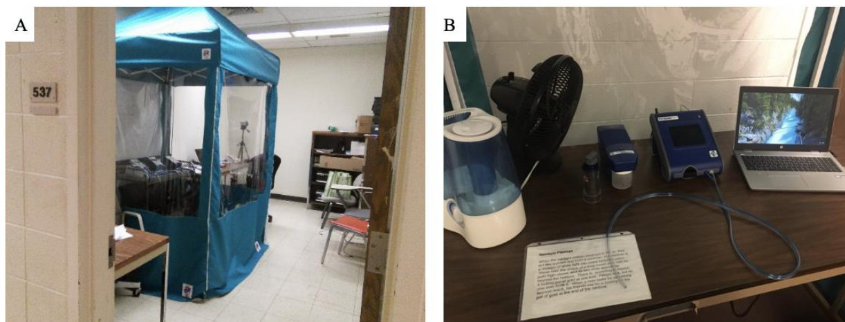
Figure 1. Fit testing equipment. Pictured from left to right: testing chamber, humidifier, fan, TSI salt generator (Model 8026), TSI PortaCount® Pro Respirator Fit Tester (Model 8038).
