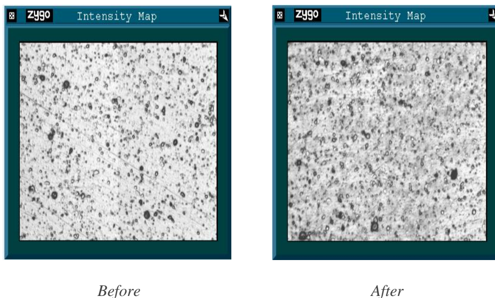
Figure 50: Intensity map collected from Tech #2 disc number 33 “Before” and “After” the pin on disc test. These maps have been collected in position 5 on the disc and so, on the unworn zone.
