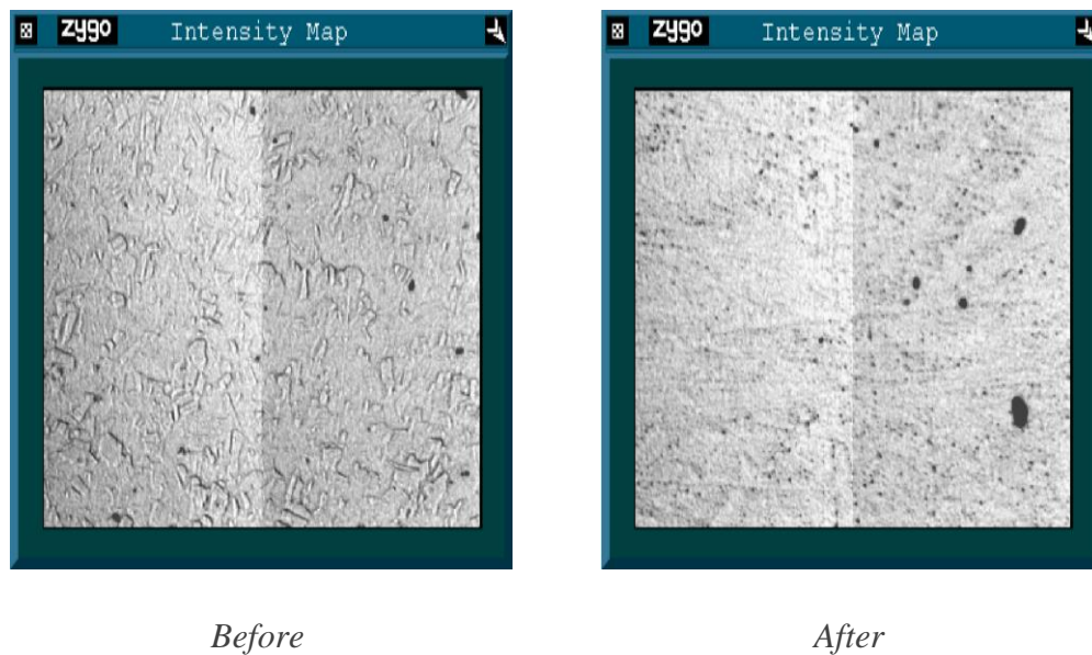
Figure 38: Intensity map collected from Tech #3 disc number 13 “Before” and “After” the pin on disc test. These maps have been collected in position 3 on the disc and so, on the wearing path.
