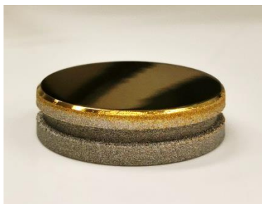
Figure 11: Details of final surface polishing.
