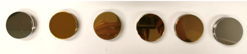
Figure 6: Different discs type. From left to right it is possible to see Uncoated CoCr disc, TiN coating, tech #1 disc, TiN coating, tech #2, TiN coating, tech #3 disc, Ag-doped TiN coating disc, Uncoated CoCr disc from the LAB.
