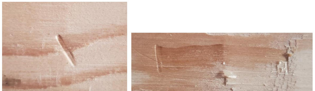
Figure 2: A representation of an impressed toolmark; pictured on the left, and a striated toolmark; pictured on the right placed on a piece of board with a screwdriver
