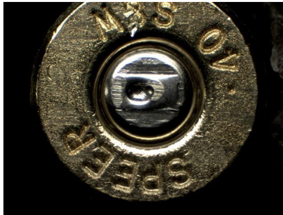
Figure 5: Pictograph of individual characteristics on a cartridge case
