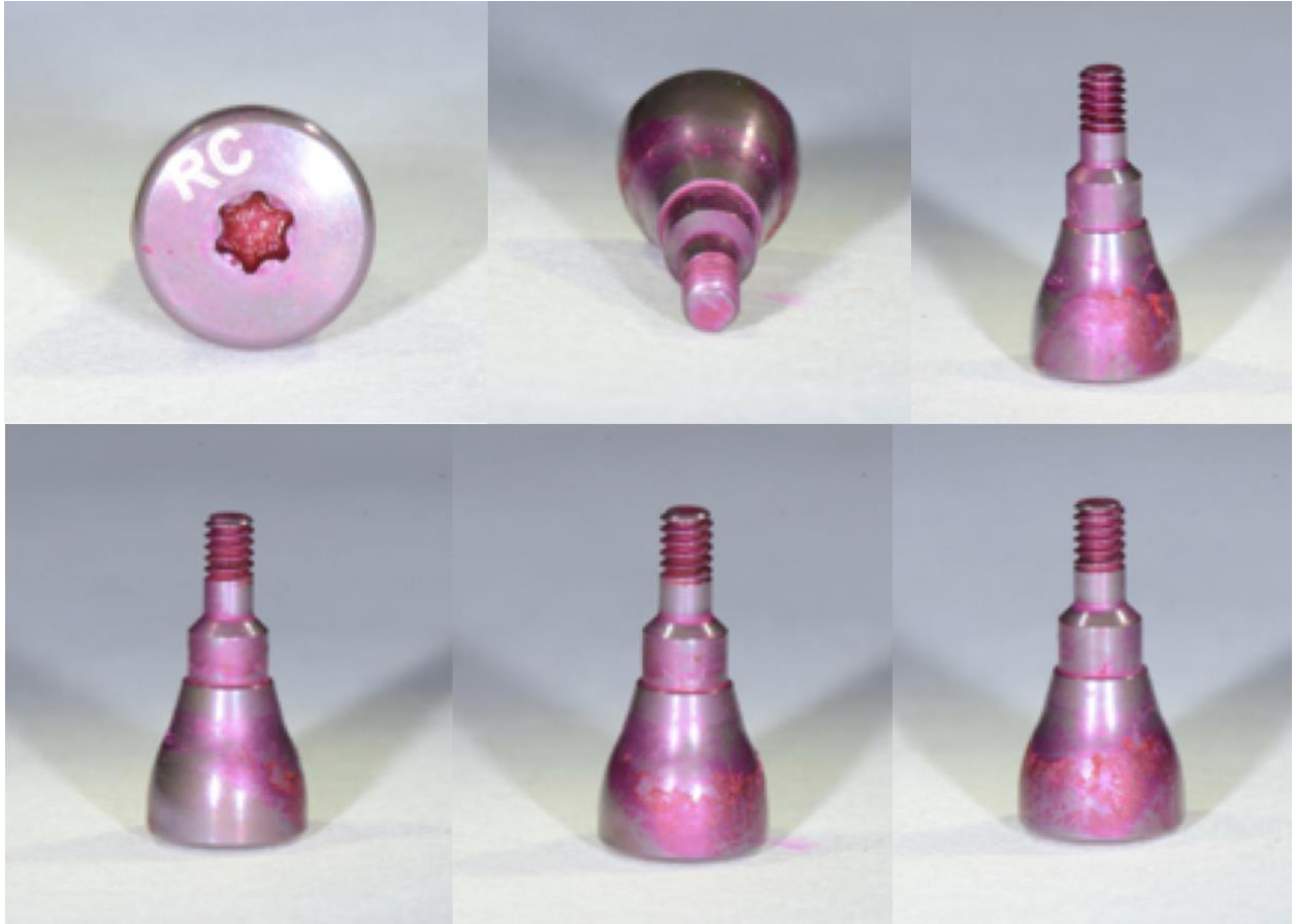
Figure 1. Images of healing abutments in test group A stained with Phloxine B demonstrating residual protein on the surface, screw threads and in the screw access
