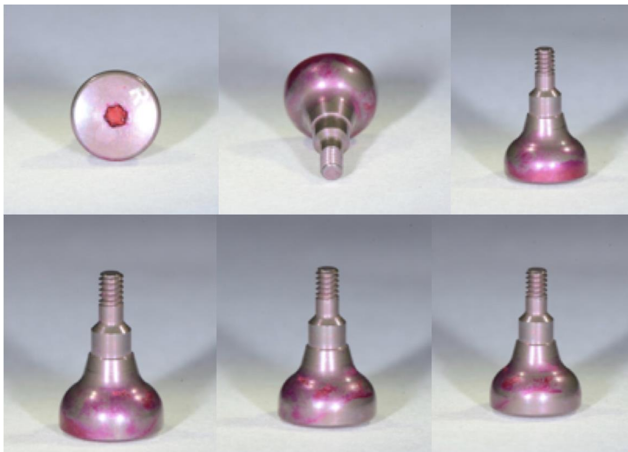
Figure 2. Images of healing abutments in test group B stained with Phloxine B demonstrating residual protein on the surface, screw threads and in the screw access
