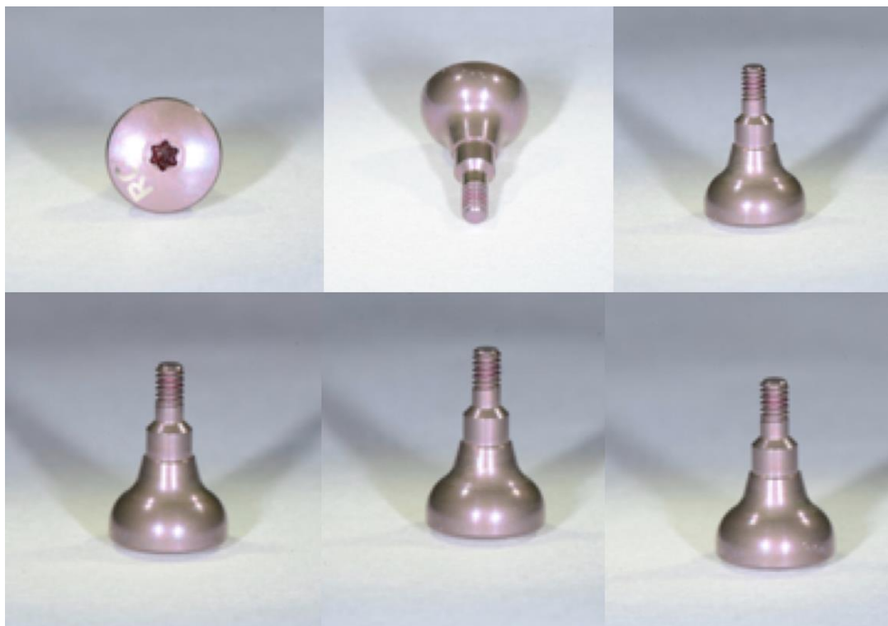
Figure 4. Images of healing abutments in test group D stained with Phloxine B demonstrating minimal residual protein on the surface, screw threads and in the screw access
