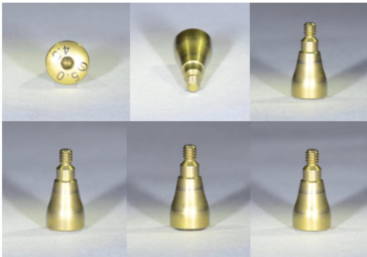
Figure 3. Images of healing abutments in test group C stained with Phloxine B demonstrating no evidence of residual protein on the surface, screw threads and in the screw access
