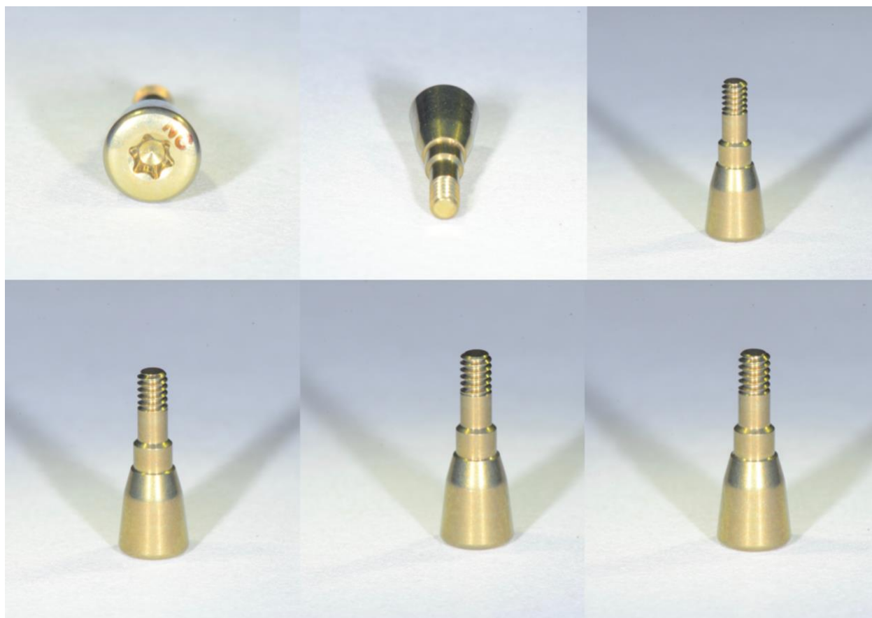
Figure 5. Images of healing abutments in test group A stained with Phloxine B demonstrating no evidence of protein on the surface, screw threads and in the screw access
