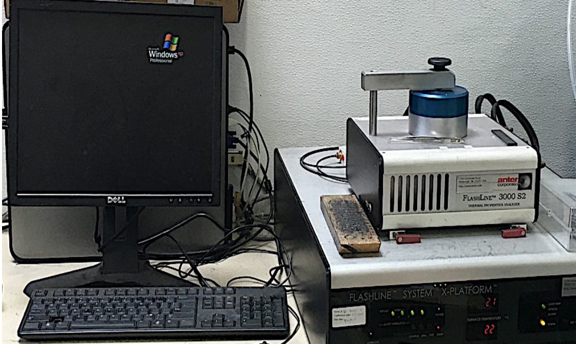
Figure 3.11: DXF-200 laser flash instrument at AllCell Technologies lab
