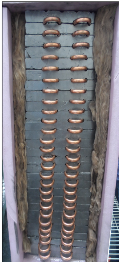
Figure 4.3: Inside view of the actual 4kWh PCC-TES structure (28 slabs stack)
