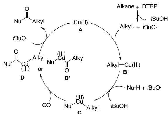
Figure 1.29 Cu-catalyzed oxidative C-H carbonylation
