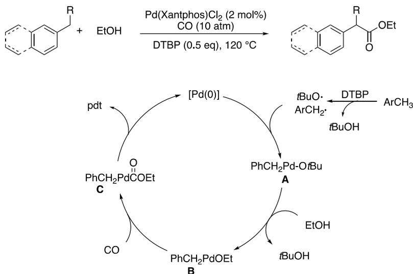
Figure 1.28 Oxidative alkoxy carbonylation of benzylic C-H bonds
