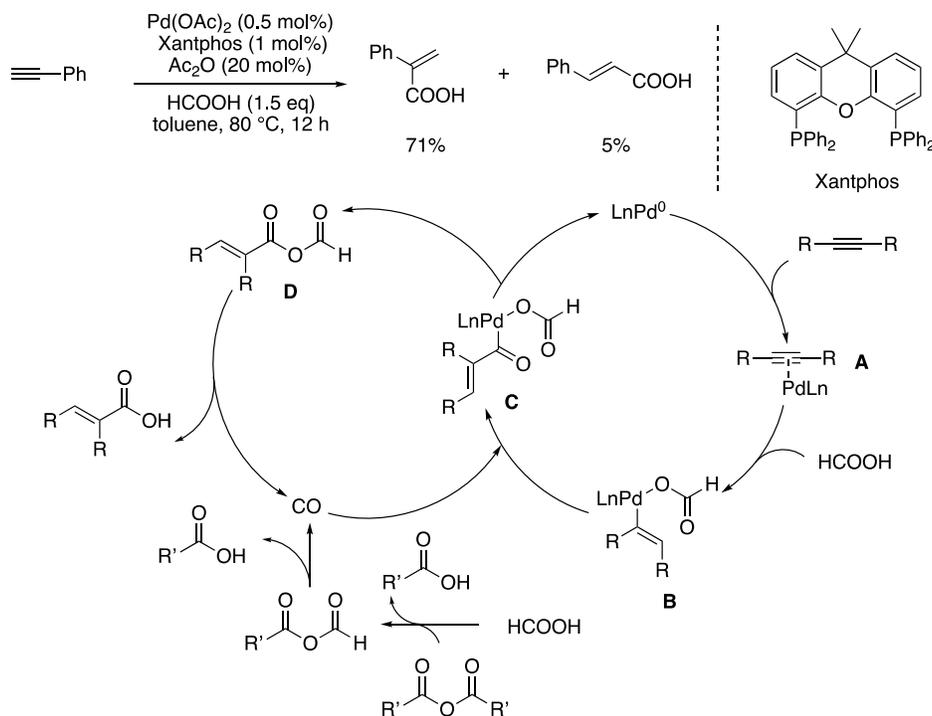
Figure 1.6 Pd-catalyzed hydroxycarbonylation of alkynes with formic acid as CO provider and proposed cycles
