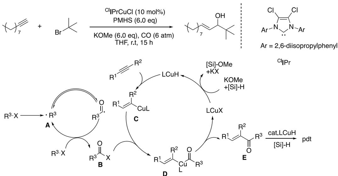
Figure 1.22 Cu-catalyzed Hydrocarbonylative carbonylation of alkynes and alkyl halides. PMHS: poly(methylhydrosiloxane)
