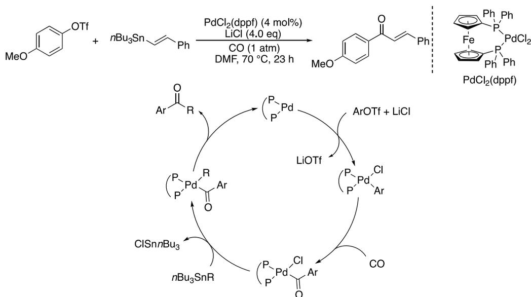
Figure 1.18 Pd-catalyzed carbonylative Stille reactions. dppf: 1,1'-ferrocenediyl-bis(diphenylphosphine)
