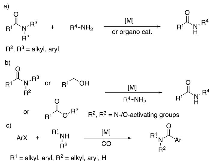
Scheme 3.2 Traditional transamidation between amides and amines. b) Cross-coupling reaction amines and amides, alcohols, or esters
