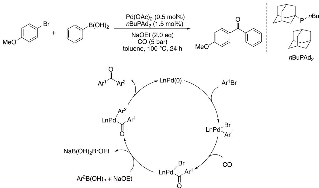
Figure 1.19 Pd-catalyzed Suzuki type carbonylation
