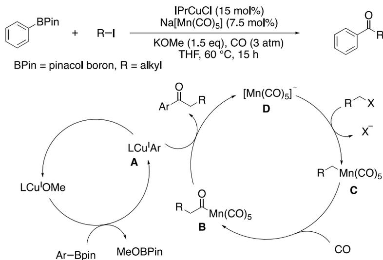
Figure 1.24 Cu/Mn co-catalyzed carbonylative Suzuki coupling
