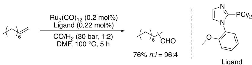
Scheme 1.2 Ru-catalyzed hydroformylation at miniplant scale
