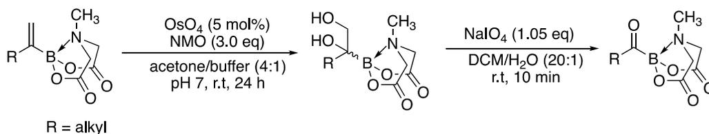
Scheme 4.5 Synthesis of MIDA-supported acylboronates from vinylboronates. NMO: *N*-methylmorpholine *N*-oxide. Buffer: aqueous monobasic phosphate buffer
