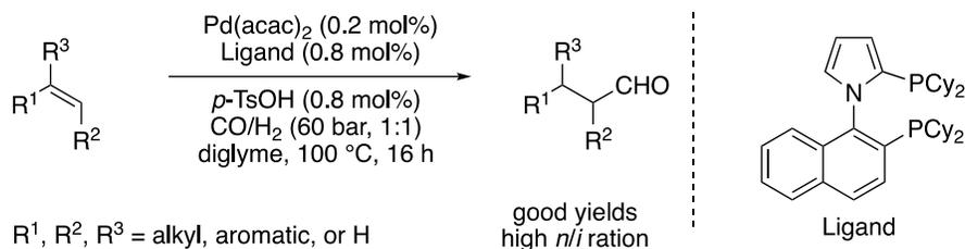
Scheme 1.5 Pd-catalyzed hydroformylation with acid additives
