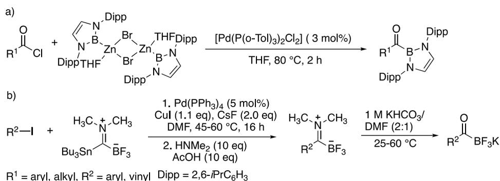
Scheme 4.6 a) Pd-catalyzed synthesis of acylboronates with acyl chlorides. b) Pd-catalyzed cross-coupling of aryl or vinyl iodides and a bifunctional reagent.
