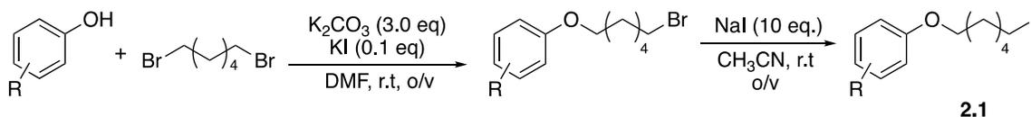
Scheme 2.11 General reaction scheme for the synthesis of alkyl iodides
