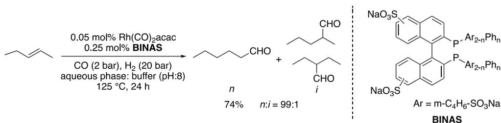
Scheme 1.1 Hydroformylation of 2-butene using Rh catalyst
