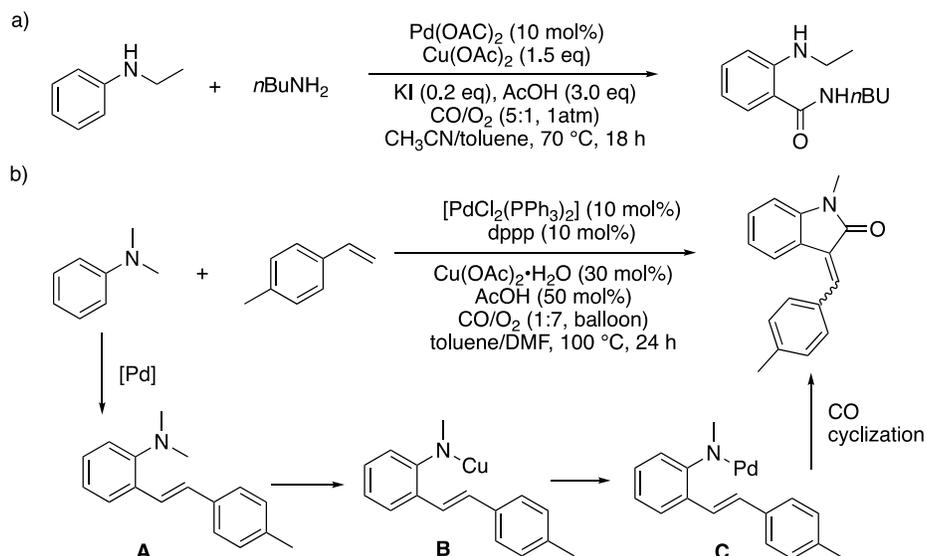
Scheme 1.27 a) Pd-catalyzed *ortho*-selective C-H carbonylation b) Pd/Cu-catalyzed cascade transformation: C-H alkenylation and N-dealkylative carbonylation
