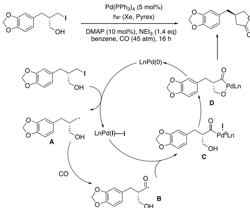
Figure 1.21 Pd/light-accelerated atom transfer carbonylation of alkyl iodides. DMAP: 4-methylaminopyridine
