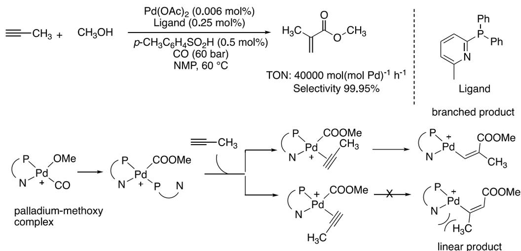
Scheme 1.17 Pd-catalyzed alkoxy carbonylation of alkynes for efficient synthesis of branched methacrylates
