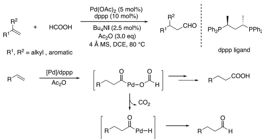
Scheme 1.6 Pd-catalyzed hydroformylation with HCOOH
