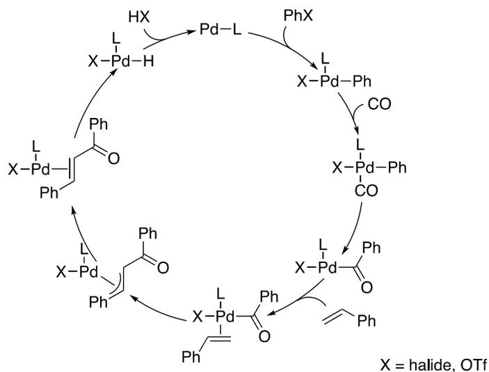
Figure 1.5 General mechanism for a palladium-catalyzed carbonylative Heck reaction
