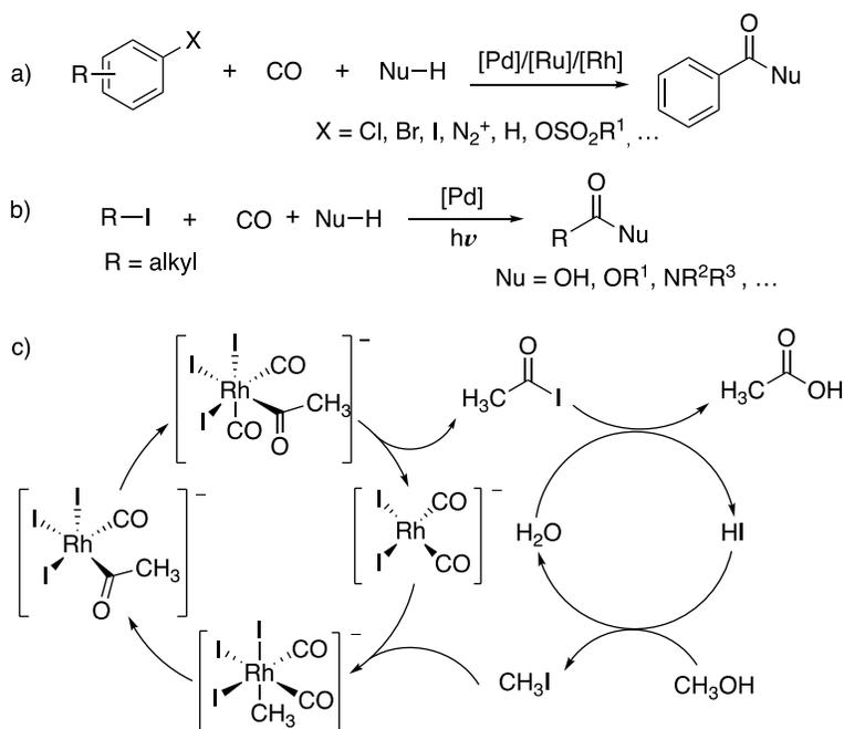
Figure 1.2 a) Transition metal-catalyzed Heck carbonylation, b) Ryu's radical carbonylation of alkyl iodides, c) Monsanto process
