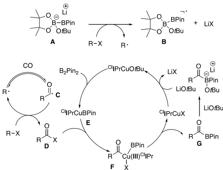
Scheme 4.11 Proposed catalytic cycle for carbonylative borylation
