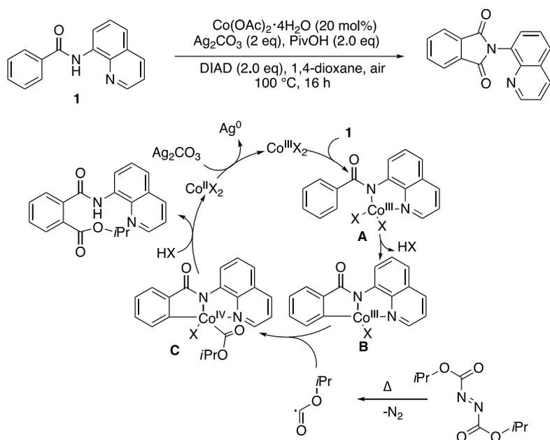
Figure 1.30 Co-catalyzed  $\text{C}(\text{sp}^2)$ -H carbonylation
