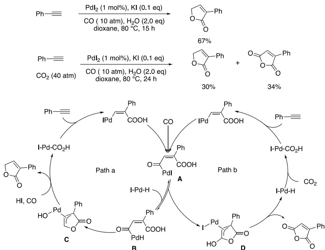
Figure 1.7 Pd-catalyzed cyclocarbonylation of alkynes with and without CO<sub>2</sub>. Path a, catalytic cycle for the formation of furanone; path b, catalytic cycle for the formation of maleic acid
