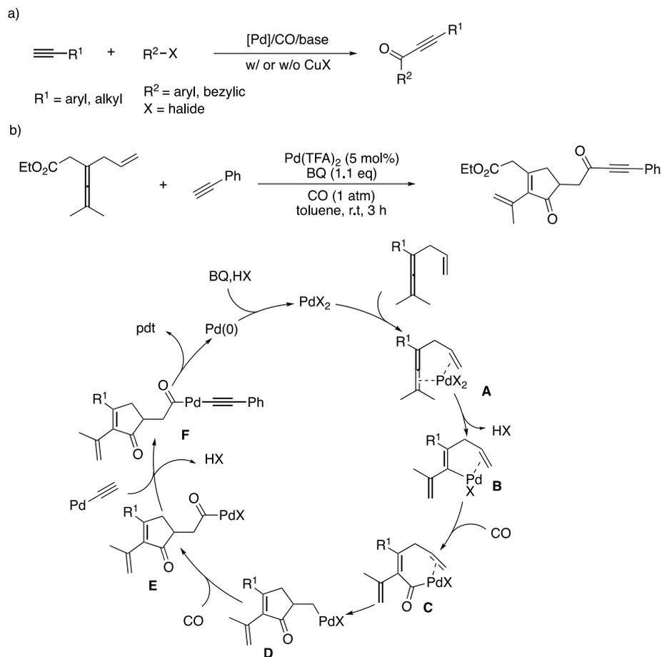
Figure 1.8 a) General scheme of carbonylative Sonogashira coupling reactions; b) Pd-catalyzed oxidative carbonylation of enallenes; BQ: benzoquinone
