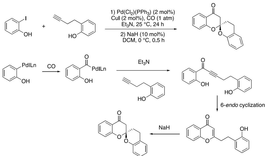
Scheme 1.19 Pd-catalyzed carbonylative Sonogashira annulation to construct spiroketals in one pot
