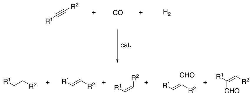
Scheme 1.14 Possible products from hydroformylation of alkynes
