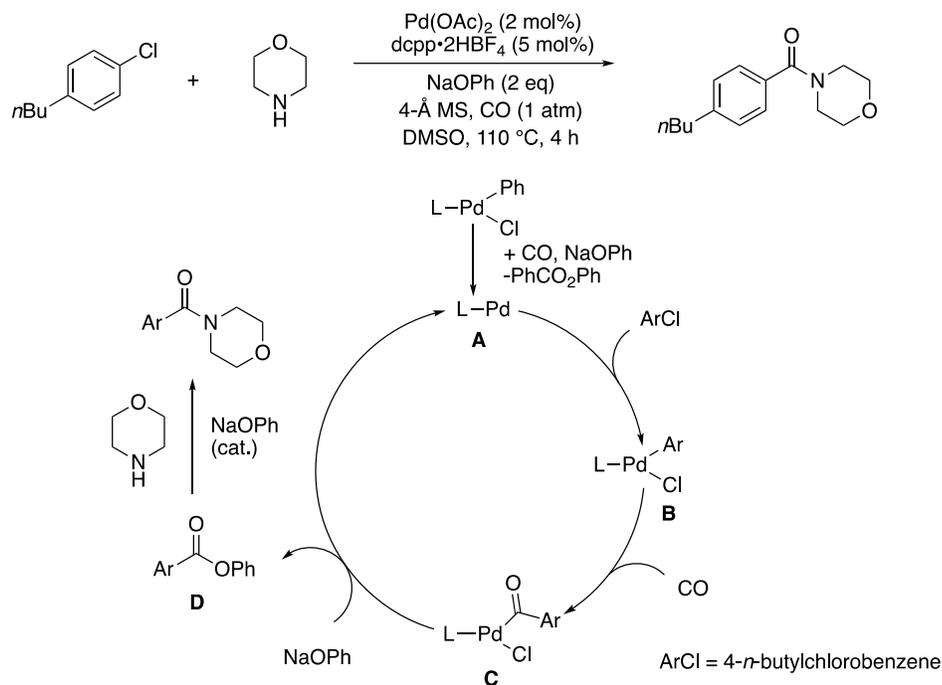
Figure 1.16 Pd-catalyzed aminocarbonylation of aryl chlorides with sodium phenoxide additive
