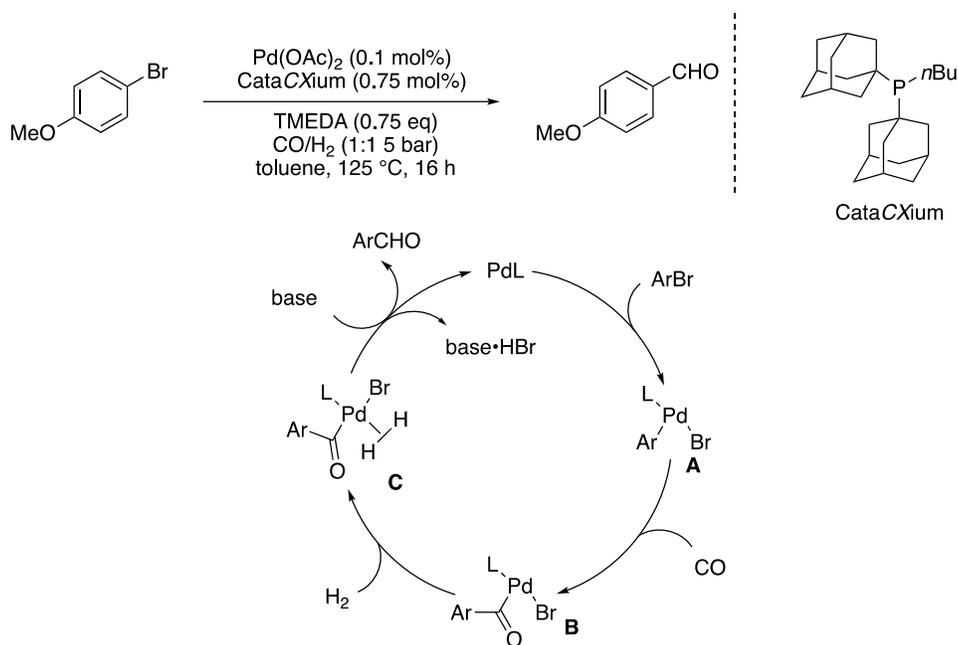
Figure 1.14 General Pd-catalyzed formylation of aryl bromide with air stable CataCXium phosphine ligand; TMEDA: tetramethylethylenediamine
