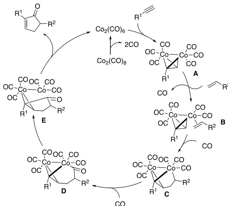
Figure 1.13 General mechanistic cycle for catalytic Pauson-Khand reaction catalyzed by  $\text{Co}_2(\text{CO})_8$
