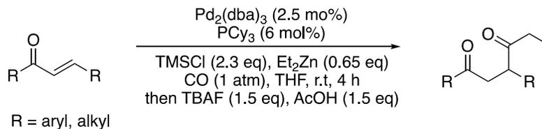
Scheme 1.26 Pd-catalyzed carbonylative Negishi reaction with unsaturated carbonyls
