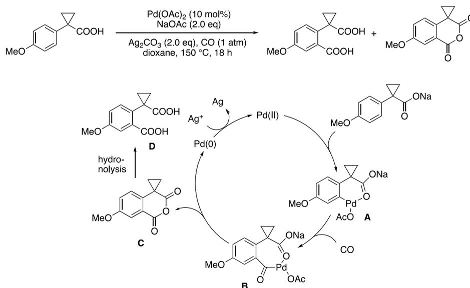
Figure 1.20 Pd-catalyzed carboxylation of aryl C-H bonds for the synthesis of 1,2 and 1,3-dicarboxylic acids
