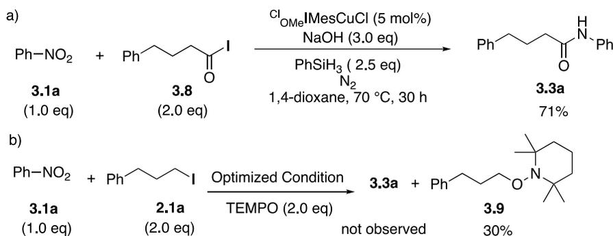
Scheme 3.8 a) Stoichiometric reaction with acyl iodide under inert atmosphere. b) Reaction with TEMPO reagent. Yield is isolated yield. For both a) and b) reactions were done on a 0.1mmol scale, and yields were determined by <sup>1</sup>H NMR with 1,1,2,2-tetrachloroethane as internal standard.
