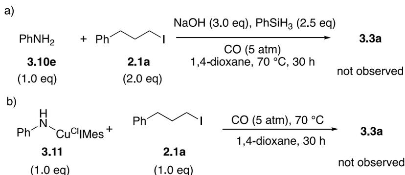
Scheme 3.9 a) Control experiments without Cu catalyst. b) Control experiment with potential copper amide intermediate. For both a) and b), reactions were done on a 0.1 mmol scale, and yields were determined by <sup>1</sup>H NMR with 1,1,2,2-tetrachloroethane as internal standard.
