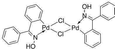
Figure 1.15 Novel dimeric cyclometallated oxime palladium catalyst for carbonylation of aryl iodides
