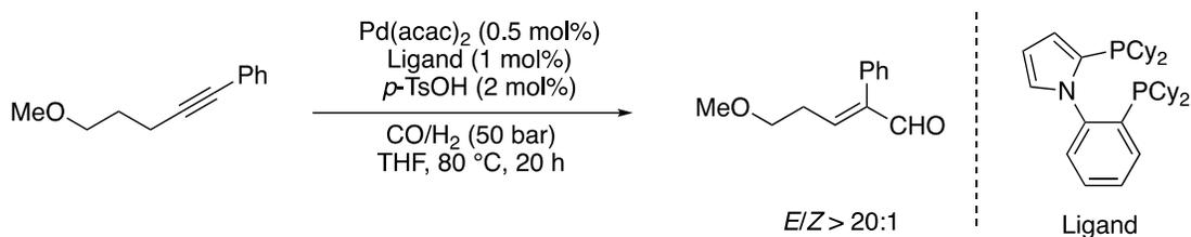
Scheme 1.15 Pd-catalyzed regio- and stereoselective hydroformylation of alkynes
