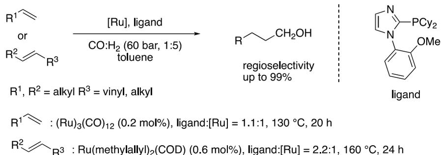
Scheme 2.2 Ru-catalyzed hydroformylation/reduction of olefins to alcohols
