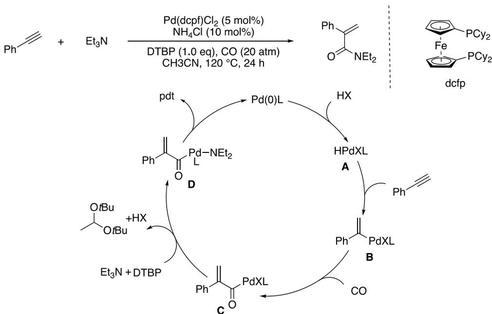
Figure 1.11 Pd-catalyzed hydroaminocarbonylation of alkynes and tertiary amines to branched amides synthesis. dcpf: 1,1'-bis(dicyclohexylphosphino)ferrocene
