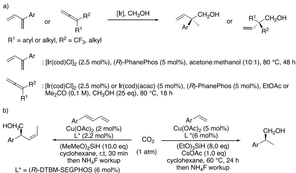
Scheme 2.3 a) Ir-catalyzed hydroxymethylation of dienes or allenes using methanol as C1 building block. b) Cu-catalyzed enantio- and regioselective reductive carbonylation of styrenes or 1,3-dienes using CO<sub>2</sub>
