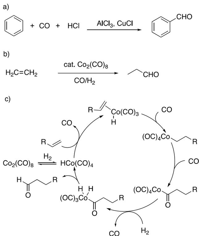
Figure 1.1 a) Gattermann-Koch reaction, b) First hydroformylation by Roelen, c) Heck and Breslow's monometallic pathway for hydroformylation by  $\text{HCo}(\text{CO})_4$  (linear product only showed here)
