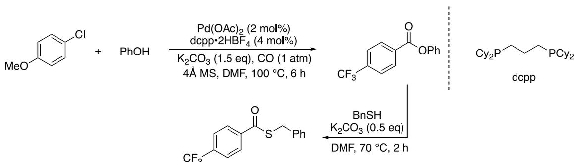
Scheme 1.25 Pd-catalyzed carbonylation of aryl chlorides to prepare phenyl esters as acyl transfer reagent
