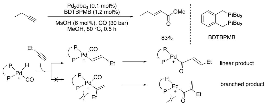
Scheme 1.18 Pd-catalyzed methoxycarbonylation of alkynes for the synthesis of linear esters
