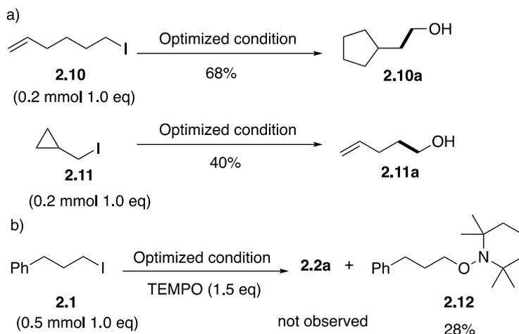
Scheme 2.8 a) Radical clock experiments. Yields were determined by  $^1\text{H}$  NMR with dibromomethane as internal standards. b) Radical trapping experiment with TEMPO reagent. Yield is isolated yield. TEMPO: 2,2,6,6-tetramethyl-1-piperidine 1-oxyl.
