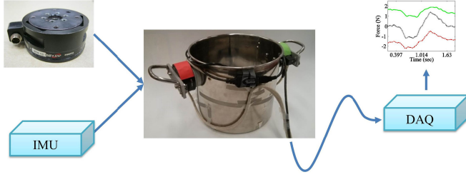
Fig. 7. Experimental setup. The force sensors are installed between the handles and the container. The IMU is interfaced with a Arduino board and placed in a box that is glued to the inside bottom of the pot. The sampled data is collected by a GUI in MATLAB.
