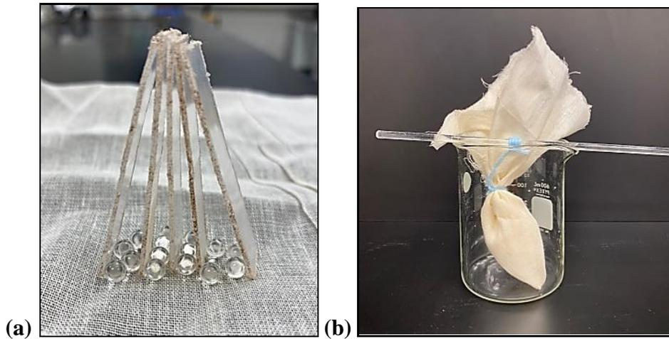
Figure 11: (a) Demonstration of five stained specimens prepared for destaining in cheesecloth and separated with glass beads to ensure homogeneous exposure of the destaining solution, (b) Each beaker contained 10 stained specimens of each material wrapped in cheesecloth, separated by glass beads and secured with a glass rod in a destaining container.
