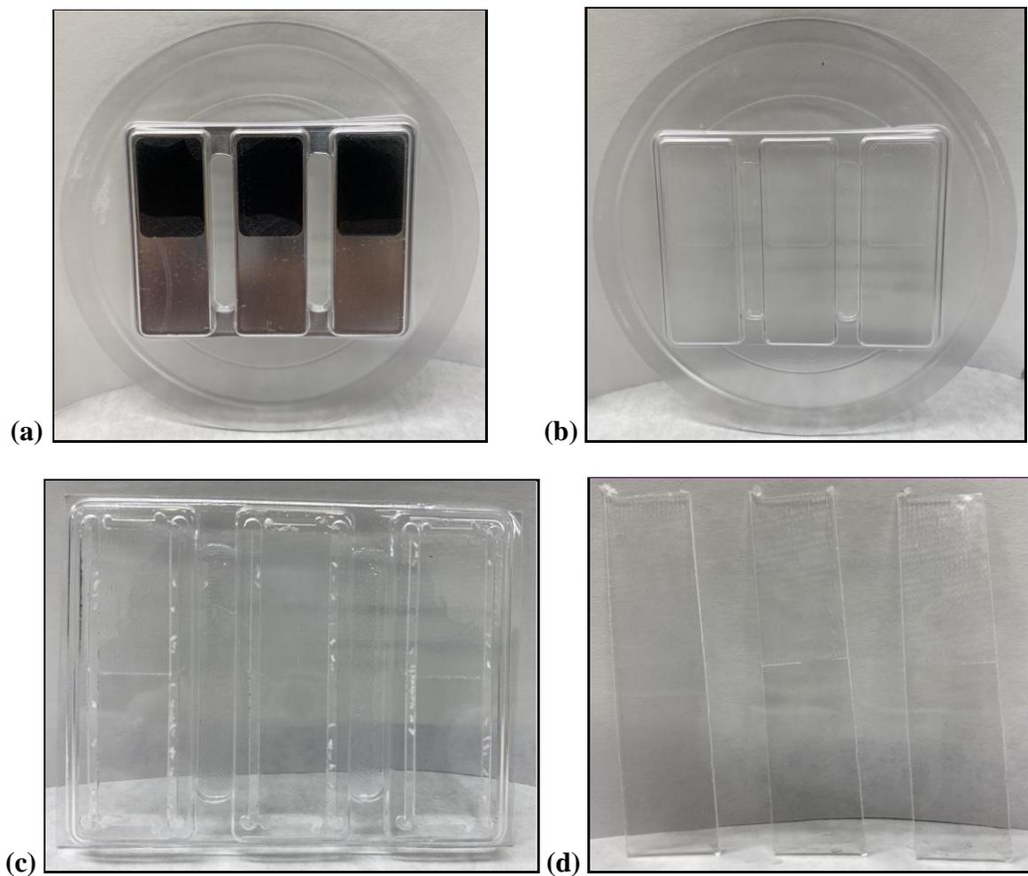
Figure 3: (a) Thermoformed material over custom stainless-steel block, (b) Thermoformed material, (c) Diamond saw cut material, (d) Specimens ready to be stained.
