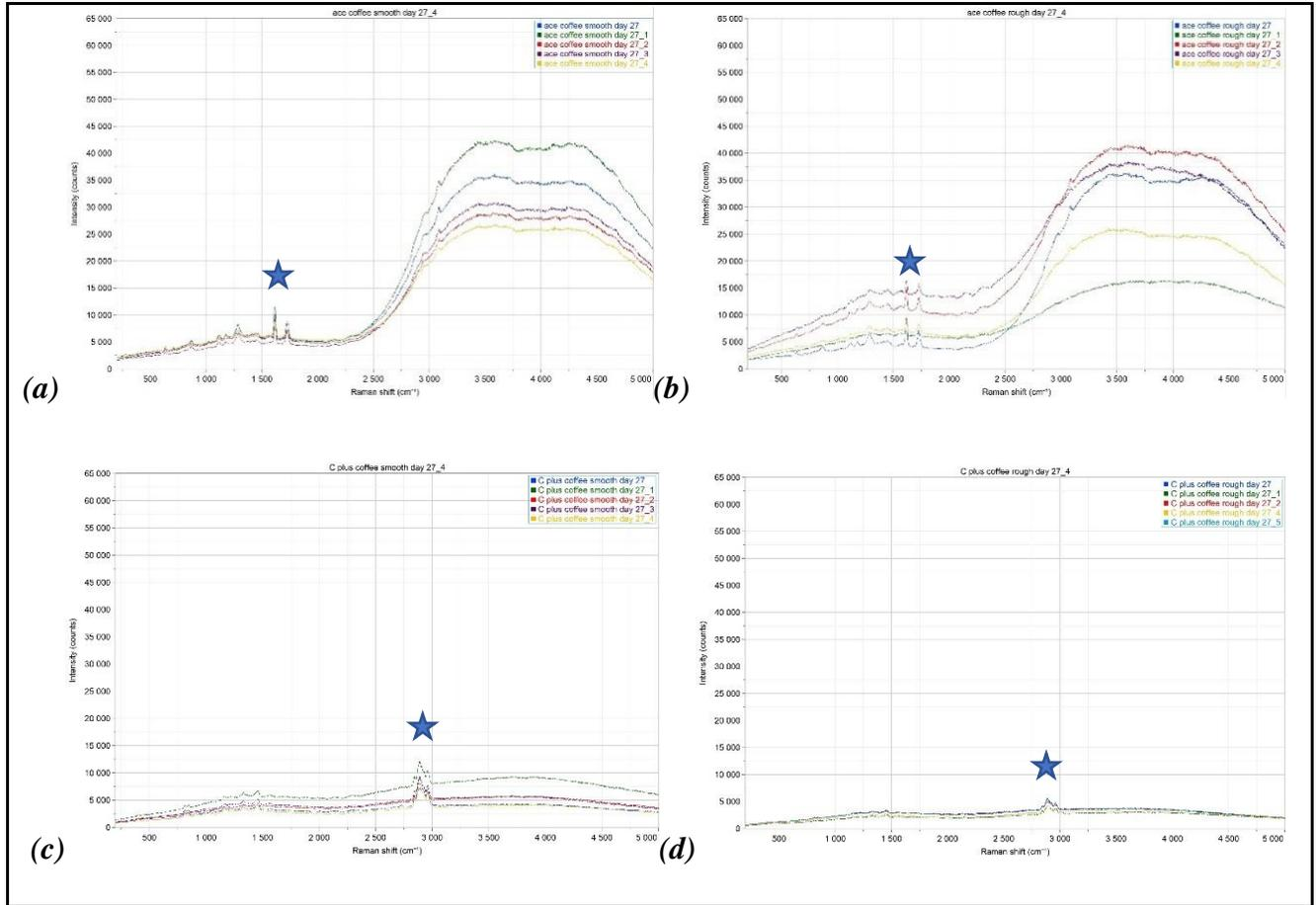
Figure 43: The patterns of composition spectrums of each material from Raman spectrometer at day 28 after staining with coffee (the end of the staining experiment). (a) Essix ACE® smooth, (b) Essix ACE® textured, (c) Essix C+® smooth, (d) Essix C+® textured
