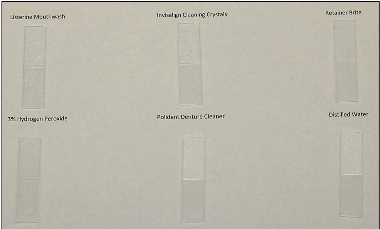
Figure 24: Essix ACE® stained with distilled water and destained with the non-ultrasonic.
