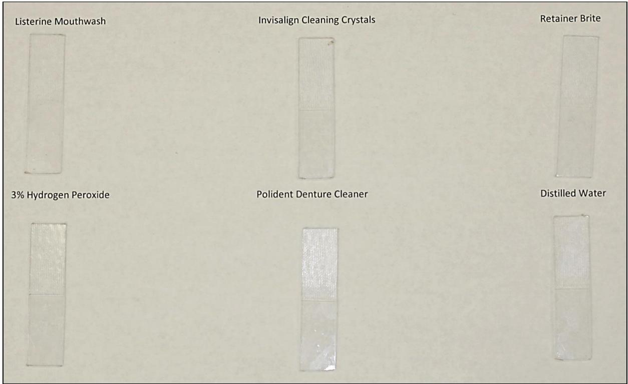
Figure 26: Essix ACE® stained with coffee and destained with the ultrasonic.
