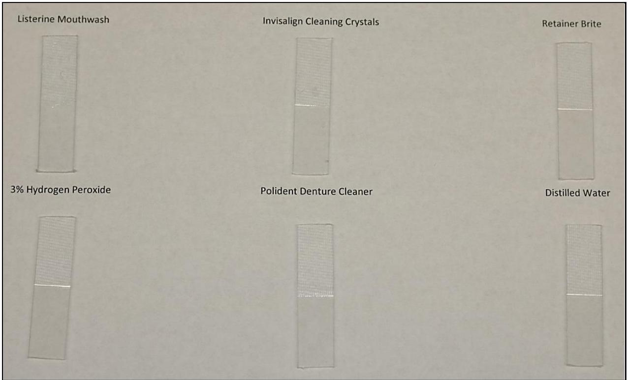
Figure 25: Essix ACE® stained with red wine and destained with the non-ultrasonic.
