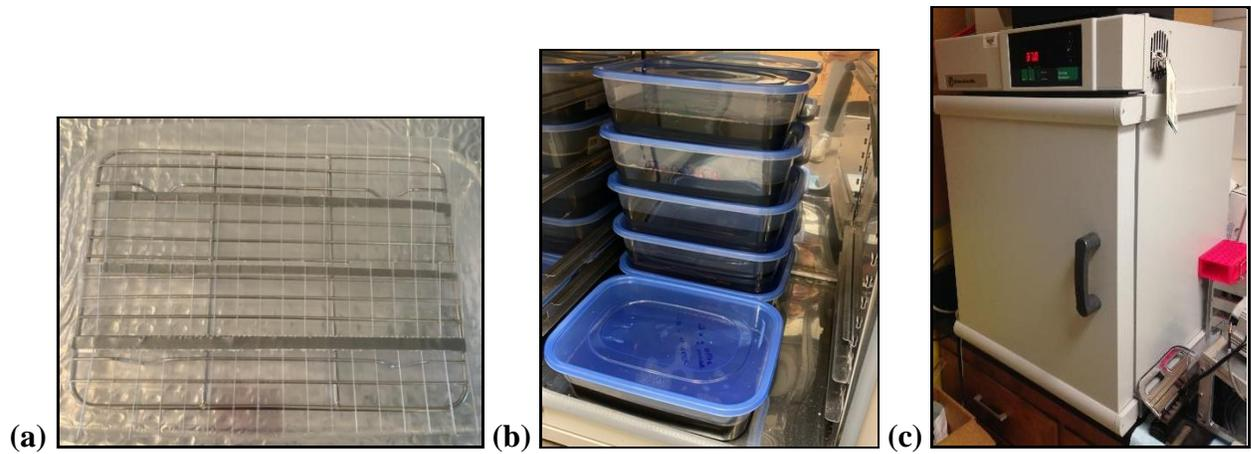
Figure 4: (a) Sixty specimens secured to on metal rack, ready for staining solutions, (b) Containers with specimens in the staining solution in the incubator, (c) 37 °C incubator.
