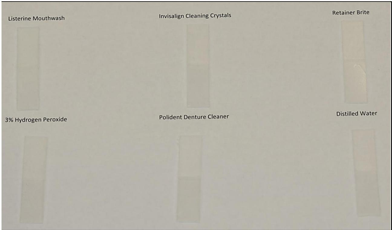
Figure 40: Essix C+® stained with distilled water and destained with the ultrasonic.
