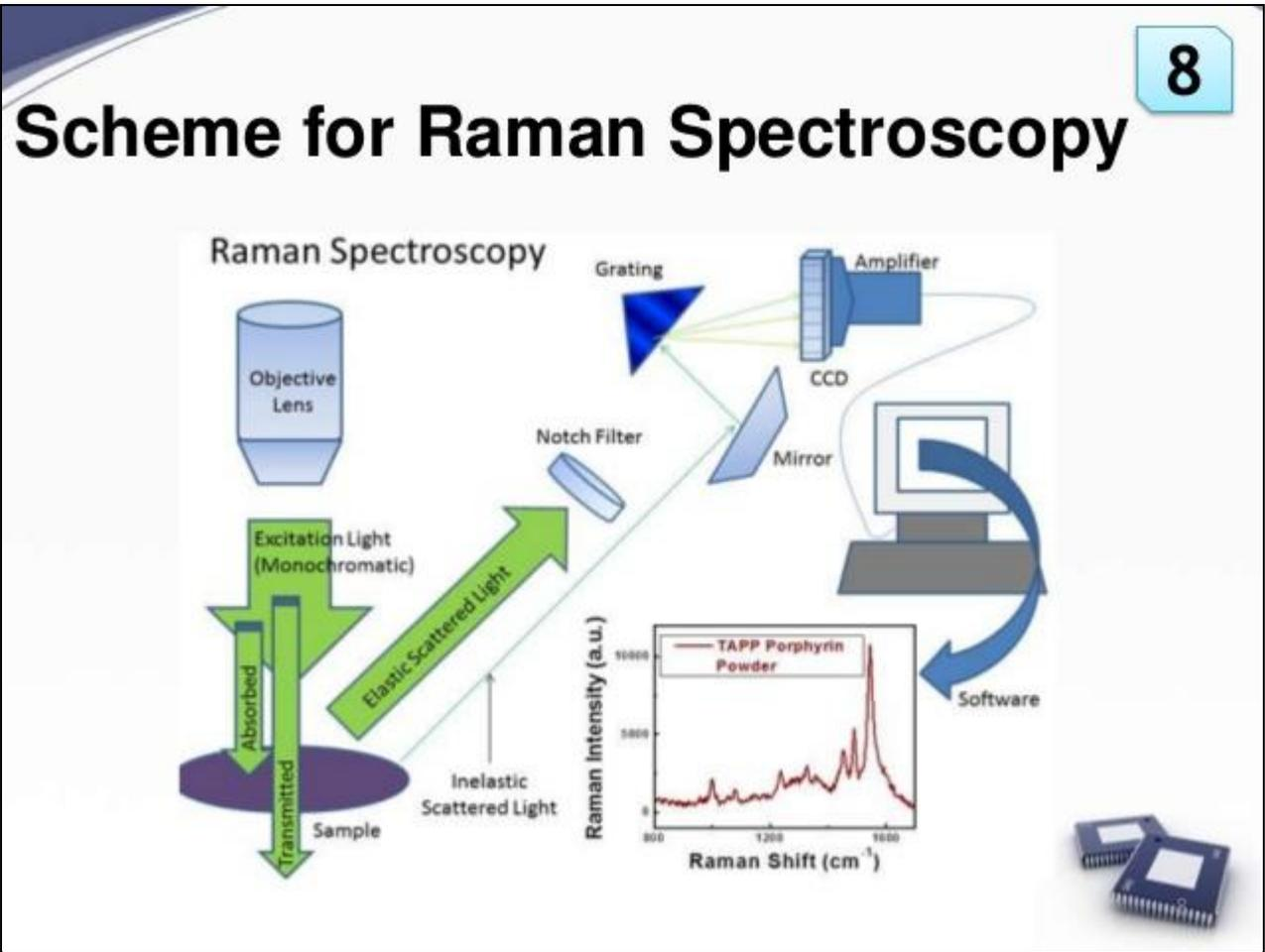
Figure 16: Raman spectrometer diagram
