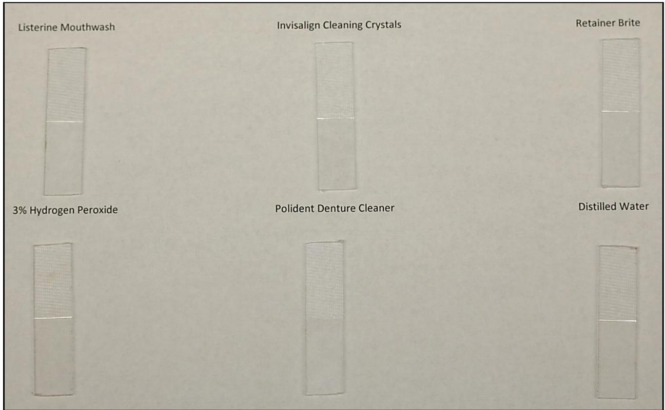
Figure 23: Essix ACE® stained with black tea and destained with the non-ultrasonic.
