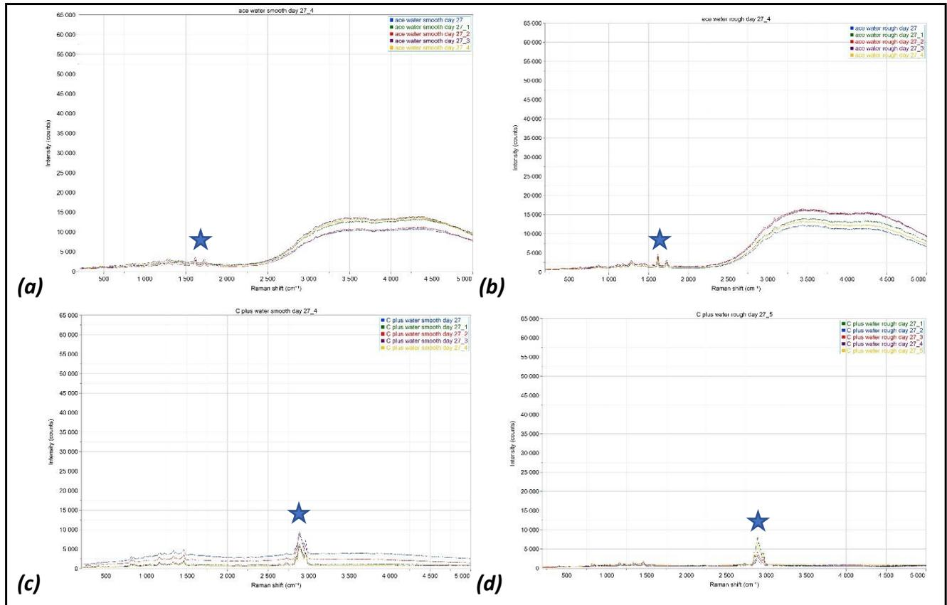
Figure 44: The patterns of composition spectrums of each material from Raman spectrometer at day 28 after staining with distilled water (the end of the staining experiment). (a) Essix ACE® smooth, (b) Essix ACE® textured, (c) Essix C+® smooth, (d) Essix C+® textured
