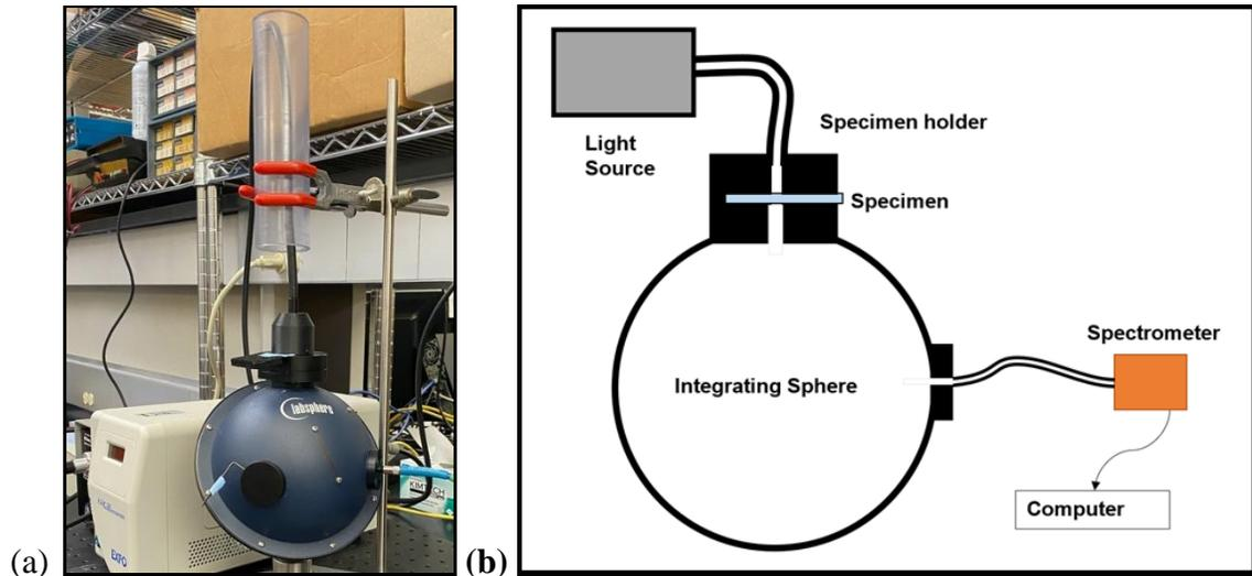
Figure 15: (a) Spectrometer Integrating sphere for evaluation of light transmittance, (b) Diagram of light transmission measurement system (Diagram courtesy of Henry Lukic, ADA Science Institute, Research and Standards).
