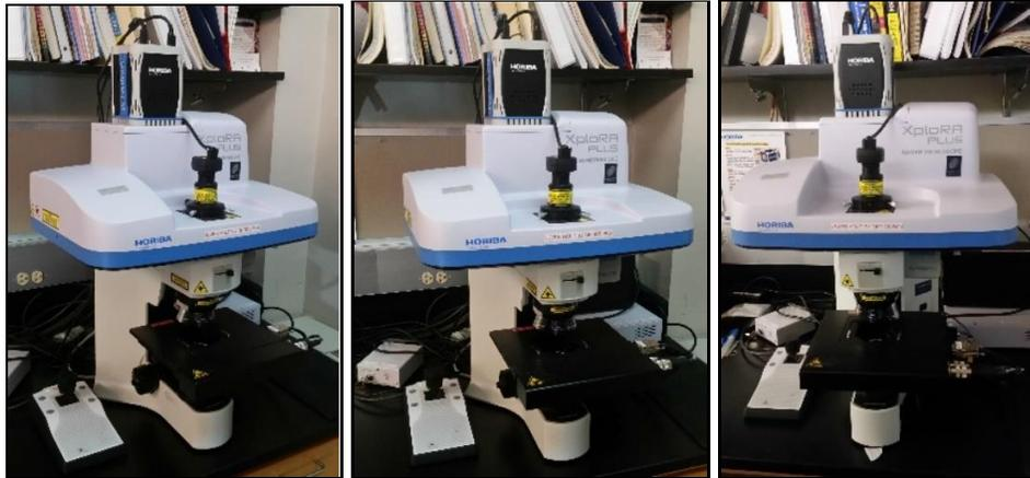
Figure 17: Raman spectrometer (XploRA Plus, Horiba Scientific)
