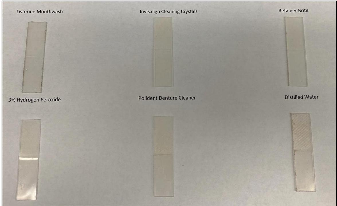
Figure 34: Essix C+® stained with coffee and destained with the non-ultrasonic.
