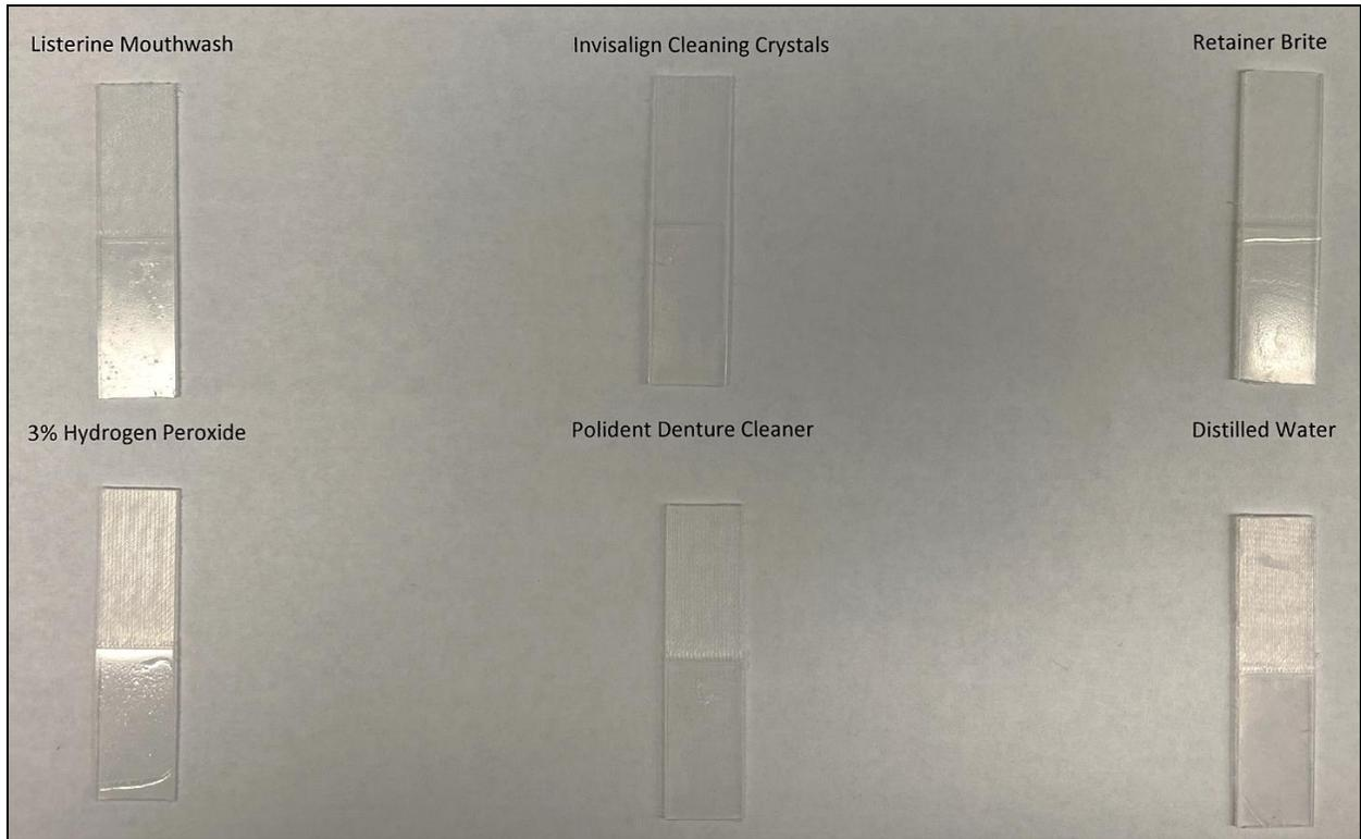
Figure 37: Essix C+® stained with red wine and destained with the non-ultrasonic.
