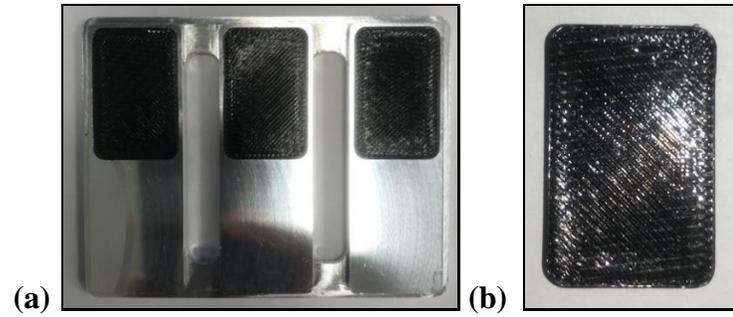
Figure 2: (a) Stainless steel block mold with two surface textures. One surface imitates a smooth surface of plaster model (bottom) and the other surface imitates the internal texture commercial models (top – black), (b) Removable polymer insert mimicking the textured surface.
