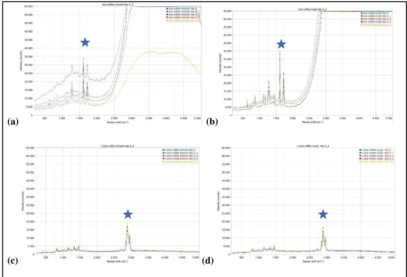
Figure 42: The patterns of composition spectrums of each material from Raman spectrometer at baseline. (a) Essix ACE<sup>®</sup> smooth, (b) Essix ACE<sup>®</sup> textured, (c) Essix C+<sup>®</sup> smooth, (d) Essix C+<sup>®</sup> textured
