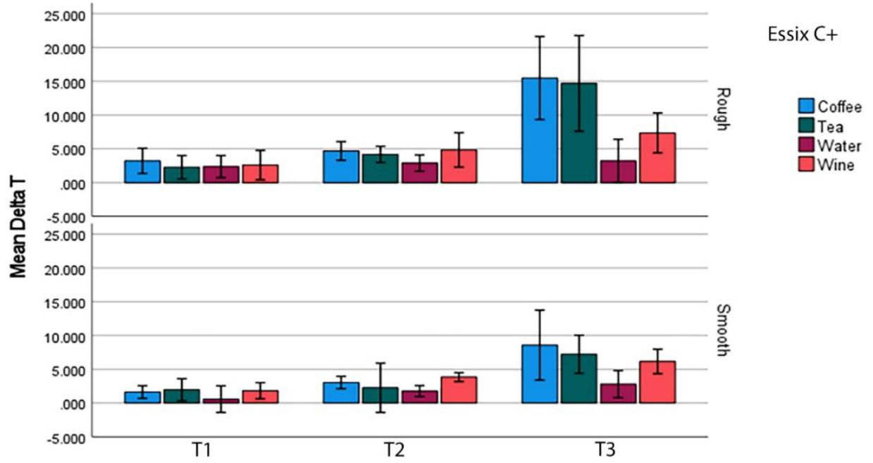
Figure 31: Mean value of  $\Delta T$  in Essix C+®
