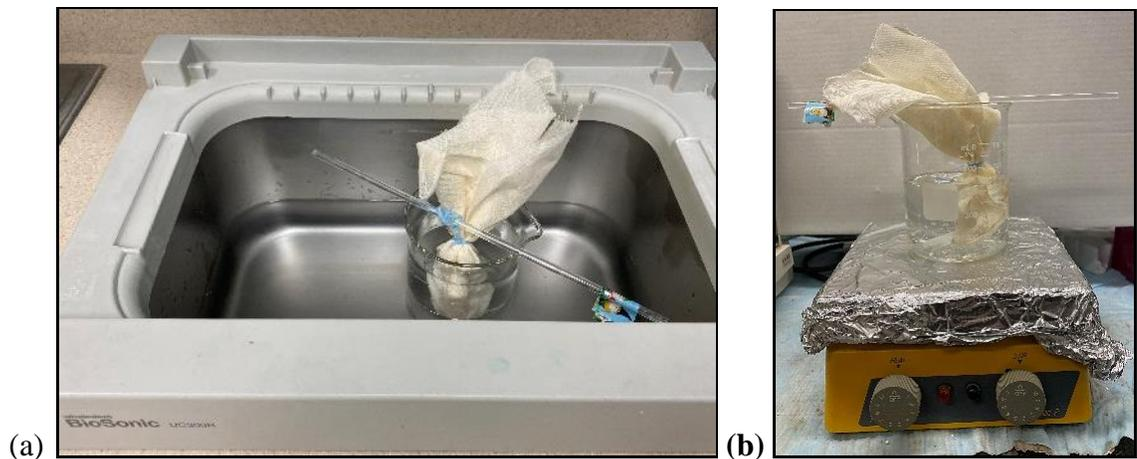
Figure 12: Destaining process settings (a) Ultrasonic cleaner unit, (b) Non-ultrasonic cleaning mean (soaked in destaining solution with a magnetic stirrer).
