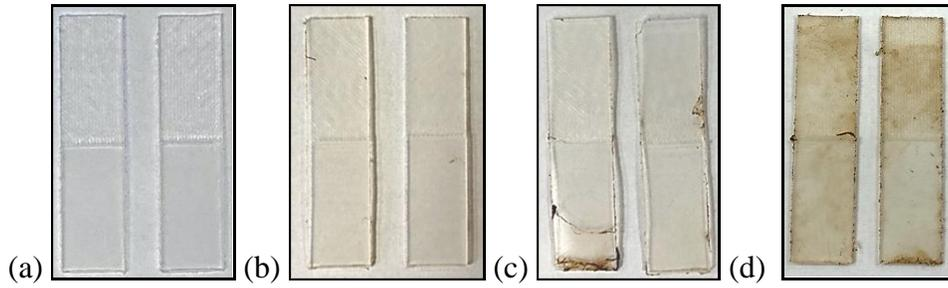
Figure 5: Essix C+® stained with coffee solution; Top section: textured, Bottom section: smooth (a) day 0, (b) day 7, (c) day 14, (d) day 28
