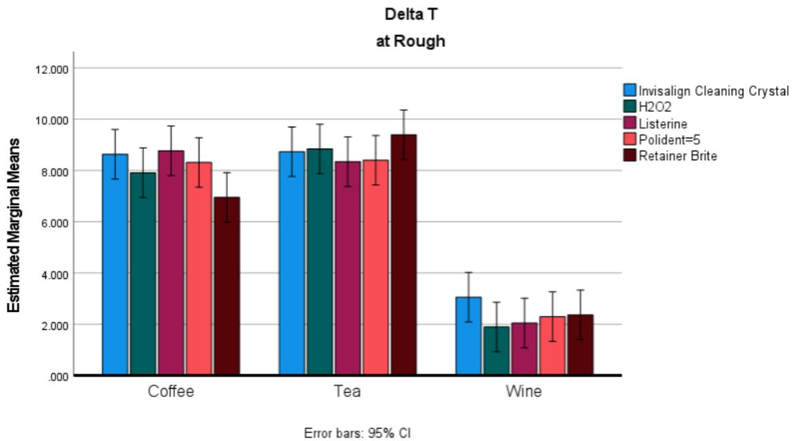
Figure 32: Comparison of Essix C+®  $\Delta T$  among destaining solutions for textured surface by type of stained specimens
