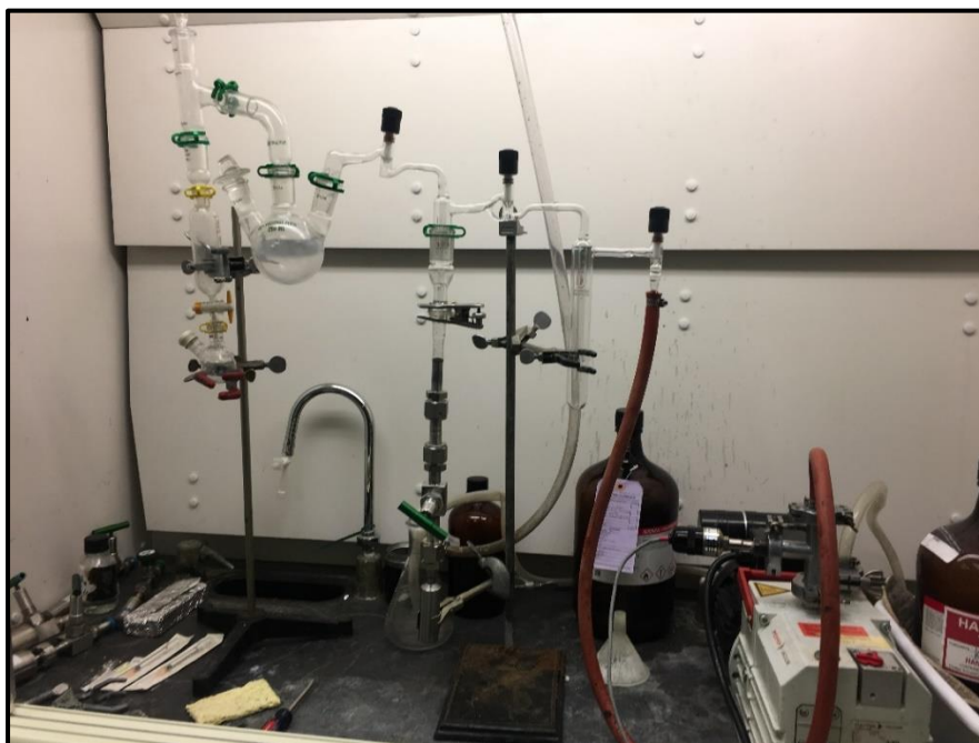
Figure 49 A photograph of the glass apparatus used for the synthesis of HCN.
