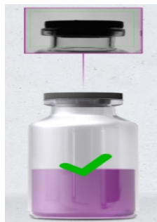
Figure 6.1: Capper Seating in Opening of the Glass Vial (Source: Heuft.(2020) [12])
