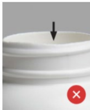
Figure 6.2: Uneven Surface on the Plastic Vial Opening (Source: (2020, July 20) [14])
