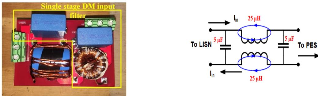
Figure 56. The DM EMI filter at the input side to suppress the DM noise peaks that are mitigated by SBC.
