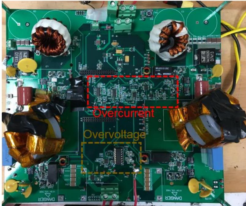
Figure A6. Illustration of the developed experimental prototype. The overcurrent and overvoltage circuits are highlighted.
