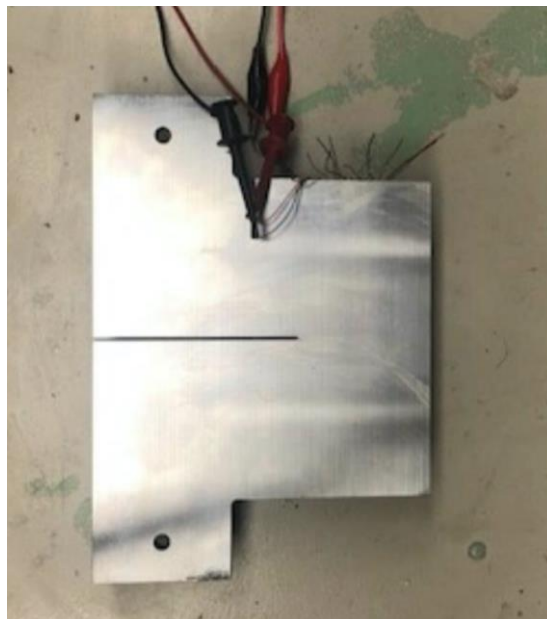
Figure 41. Actual modified steel compact tension geometry.
