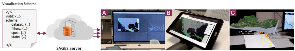
Figure 11: The visualization declaration scheme can span different devices for rendering: (a) large display, (b) tablet, and (c) HoloLens.
